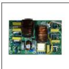
⑤ Power filter board
